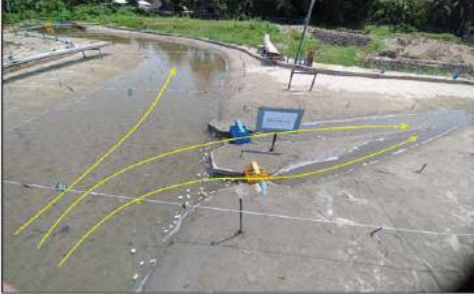
Figure 3: Flow condition at and around the regulators for average discharge in test T3 (২৫-০৪-২০২৩ খ্রিঃ)
