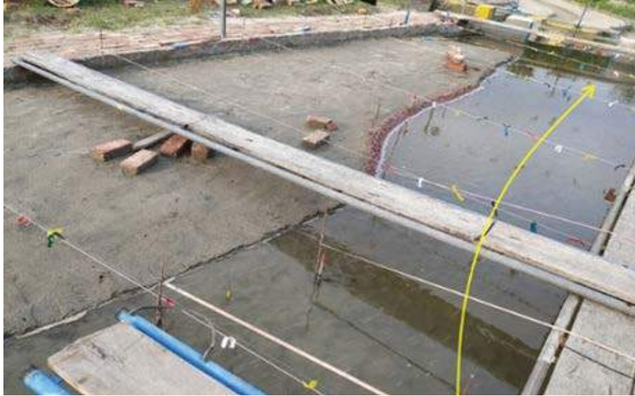
Figure 4: Occurrence of bank erosion along the left bank of Brahmaputra River under base condition in test T1 for 100 year discharge (২০-০৫-২০২৩ খ্রিঃ)
